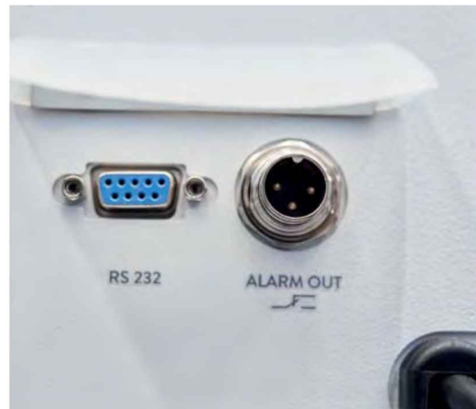
Standard-issue RS 232 interface and alarm contact
